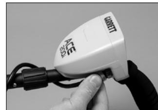
Note: The arm cuff can be adjusted by removing the screw on the bottom and moving it to the other hole.
