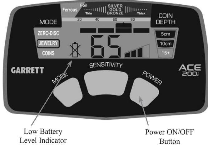
**Power ON/OFF**—Press this button to turn power ON or OFF.
