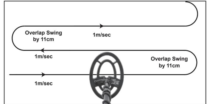
In order to fully search an area, overlap the swings of your searchcoil by half the length of the coil (about 11cm). Sweep the searchcoil in a straight line or with a slight arc at a sweep speed of about 1m/sec.
