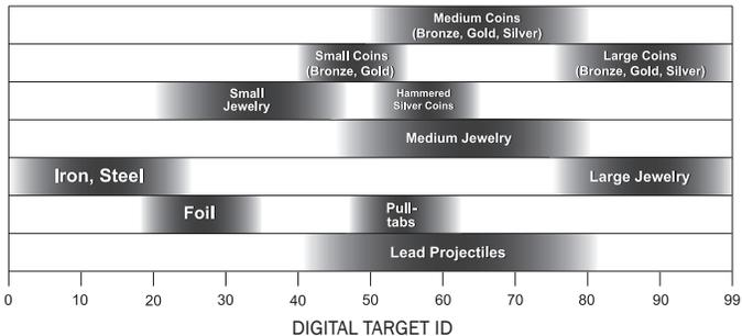
Target ID can vary widely based upon the target's size and thickness because small, thin pieces of metal cannot conduct electrical current as well as thicker pieces of metal. In addition, mineralized soils can cause Target ID errors, especially for small targets.
