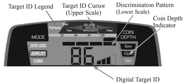
**Target ID Legend**—Works with the Target ID Cursor to indicate a target's probable identity, with Ferrous (iron) targets at the left, non-ferrous targets that are thin or have low conductivity in the middle, and thick or high conductivity targets (e.g. thick silver) at the right.
