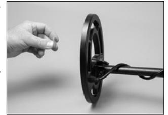
Once you have determined how your test targets register on the Target ID during bench tests, test them in the soil. Bury your targets at recorded depths to create a "test plot." Note how various targets read based upon whether they are lying in the ground flat or at various angles.
