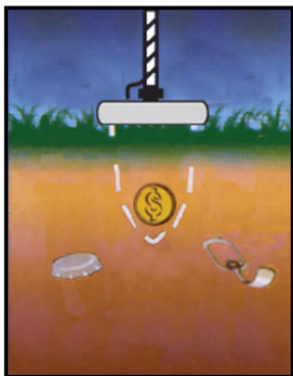
The magnetic field of a small searchcoil is not as deep as that of a large coil, but is more concentrated
