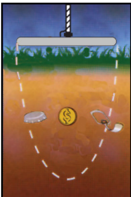
The magnetic field of a small searchcoil is not as deep as that of a large coil, but is more concentrated
